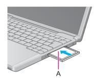
Simply slide the PC Card right-side-up until it snaps into place. Refer to the operating instructions of each card on how to insert the card. After the card is inserted, bend the eject button (A).
